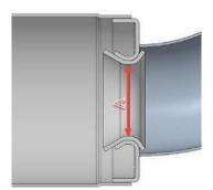
A steel ball with a 28.0mm diameter or solid flat plate measuring 28.0mm and 1.5mm thick **must not** pass through Section "A" and
